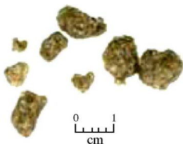
Fig. 4. Clumps of bees wax/sand from solid/liquid ratio 50/50 residence time 120 min.
