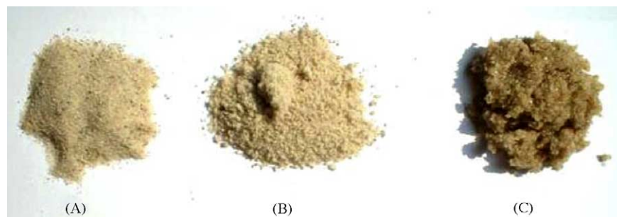
Fig. 1. (A) Clean sand; (B) bee's wax 10% contamination; (C) S341, 10% contamination.
